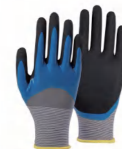
NBR 165 EN388:2016 4131X 15G nylon shell nitrile sandy double coated gloves (half/palm)
